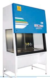
CytoFAST Elite and TOP Cytotoxic Safety Cabinets belong to the latest generation of laminar air flow systems manufactured by Faster.
